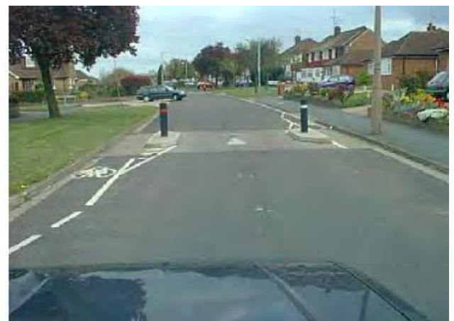
Figure 10 Examples of the traffic calming solution: pinch points
