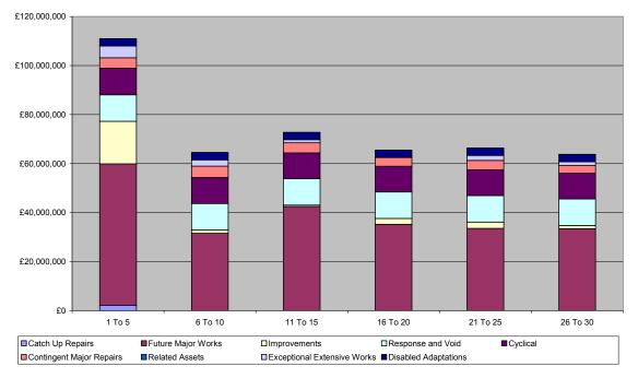
The high cost requirement in years 1 to 5 reflects the need to undertake catch-up repairs and an improvements programme. The lifecycle repeats of some components occur within the 30 year period (e.g. boilers every 15 years).
